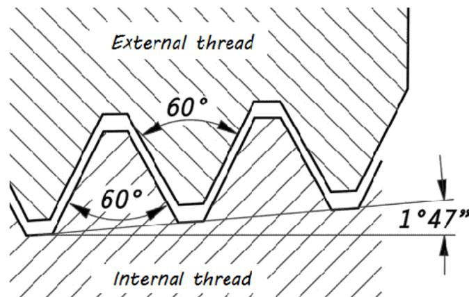
NPT threads are designed to work in conjunction with a lubricant or PTFE tape, commonly referred to as Teflon tape. The use of lubricant or PTFE tape
